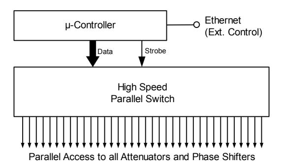
All attenuator and phase shift modules are directly connected to a register set and therefore all switch are triggered at almost the same time  $(\pm 20 \text{ns})$  up to 4000 times per second.
